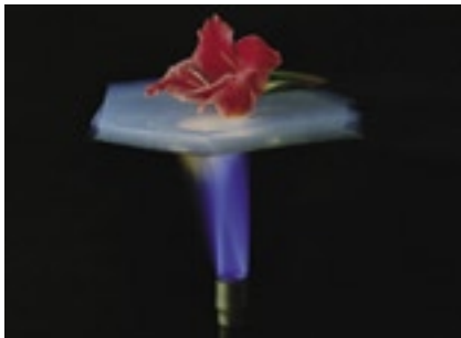
Figure 2.4: An example of an efficient insulator: an inorganic aerogel protecting a flower from a flame 10 .
