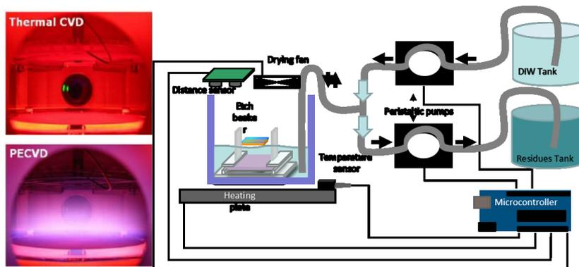
Figura 20 Scheme of the automatic transfer system for graphene and other 2D crystals.
