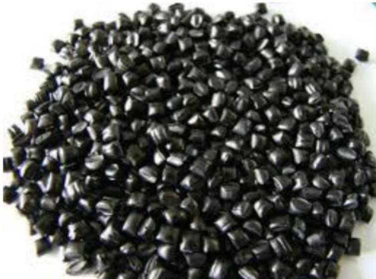
*Figura 29 Graphene polymer composite.*
